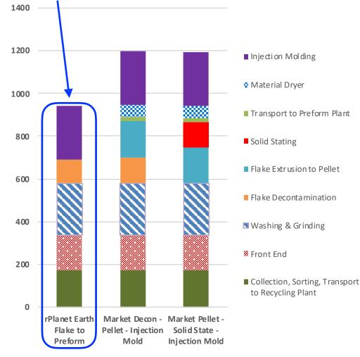
We will not pelletize the decontaminated rPET flake which not only results in less energy usage, but it also eliminates an entire heating and melting step thereby avoiding unnecessary PET degradation.
