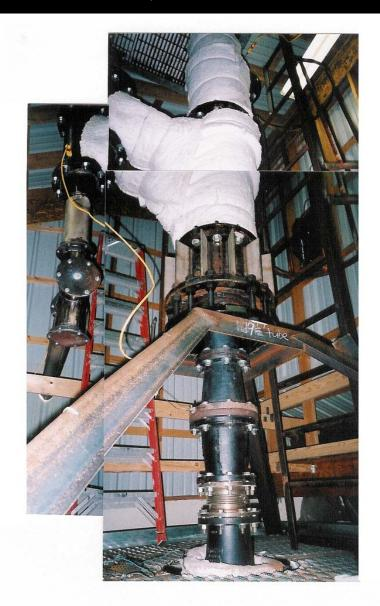
Novel two-phase gasifier On-farm energy Conversion of gas into liquid transportation fuels
